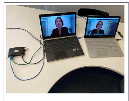
Set up two laptops and connect both to an Ethernet switch.
