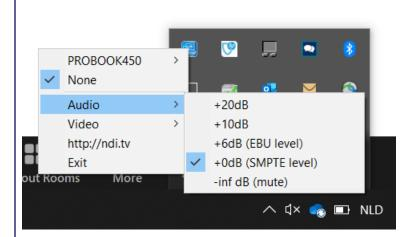
If you want to turn up the volume of the original meeting, adjust the microphone level in QuaQua. Or go to the 'NDI Webcam Input' and adjust the audio level.
